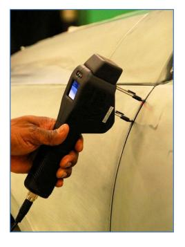
**Design** - The contoured pistol-grip handle makes the HS306 easy to hold and intuitive to use. A simple pull of the finger trigger, which is located under the handle, starts the scanning process; and when the scan and measurements are complete, a green LED signals the operator to release the trigger.
